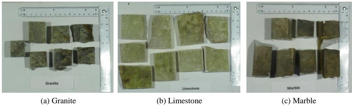
Figure 3. Masonry stone samples for greyscale imaging analysis
