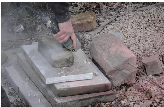
Figure 1. Cutting samples from original stones
