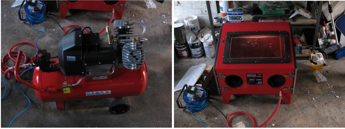
Figure 1: Air compressor and enclosed cleaning chamber
